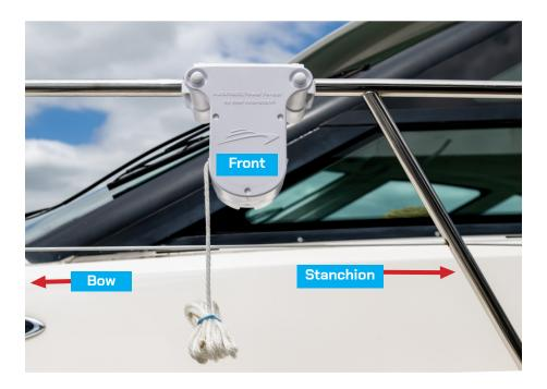
Tighten the bolts only **lightly** to allow clamp movement along the railing during the installation:
