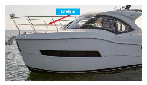
Make sure the lifeline is fully tightened and doesn't interfere with the fender's movement.
