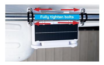
Install remaining Port, and then all Starboard AFs in the same manner. In a starboard installation the AF is left to the fender, towards the stern:
