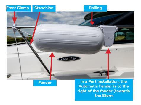
Install the front clamp on the railing infront of the stanchion, Do not skip a stanchion :
