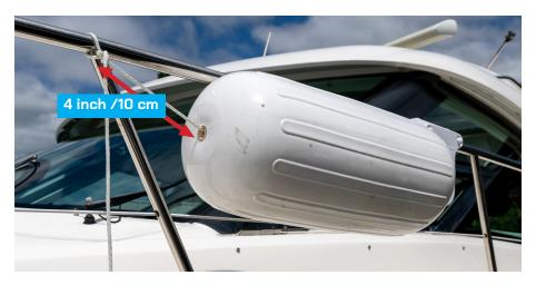
Too little of a distance between the knot and the fender may cause the fender to get stuck and not deploy properly. If the fender is stuck, the rope may get tangled.
