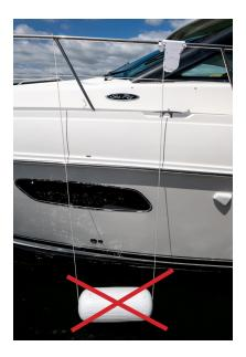
If the fender is horizontal, lift and deploy again.
